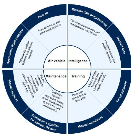
Figure 2: The Eight Elements of the F-35 Air System
