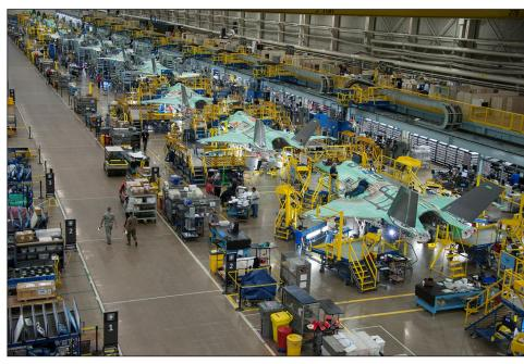
Figure 11: F-35 Aircraft in Final Assembly
