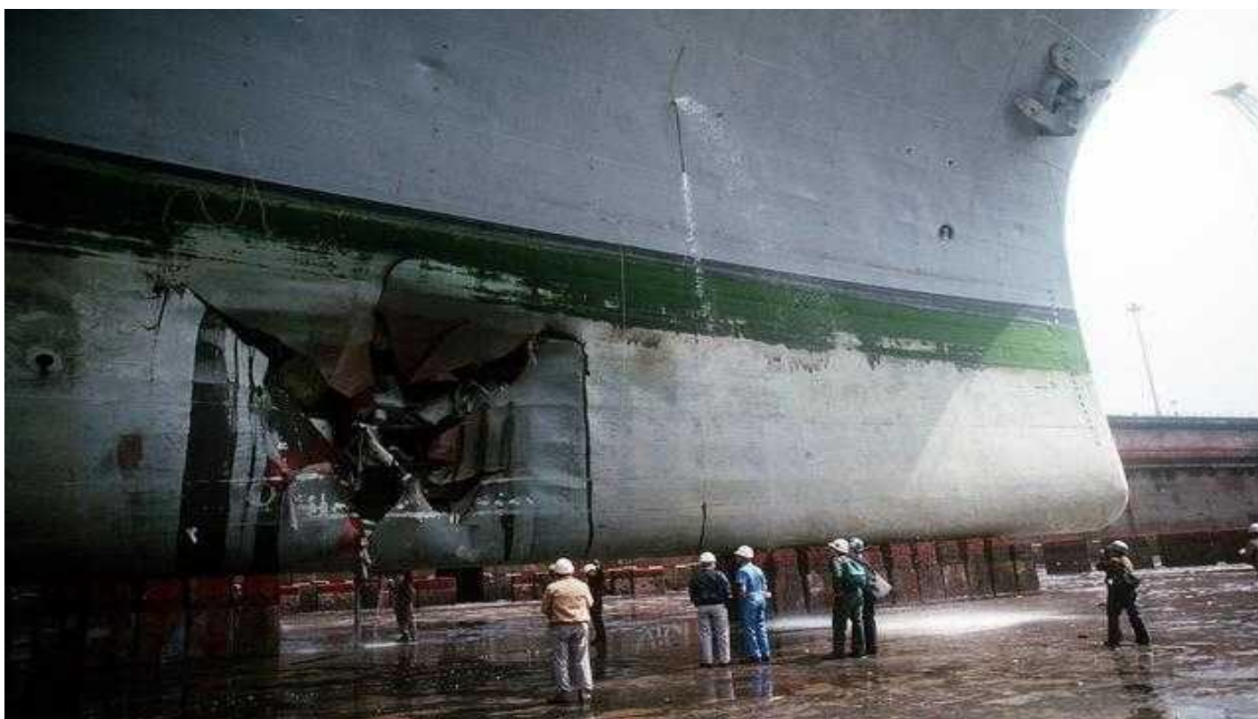
Figure 2: Sea Mine Damage to the U.S.S. Tripoli in the Gulf War
