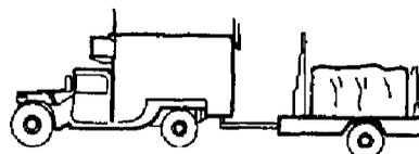
HMMWV with ground control station      10 Kw generator
