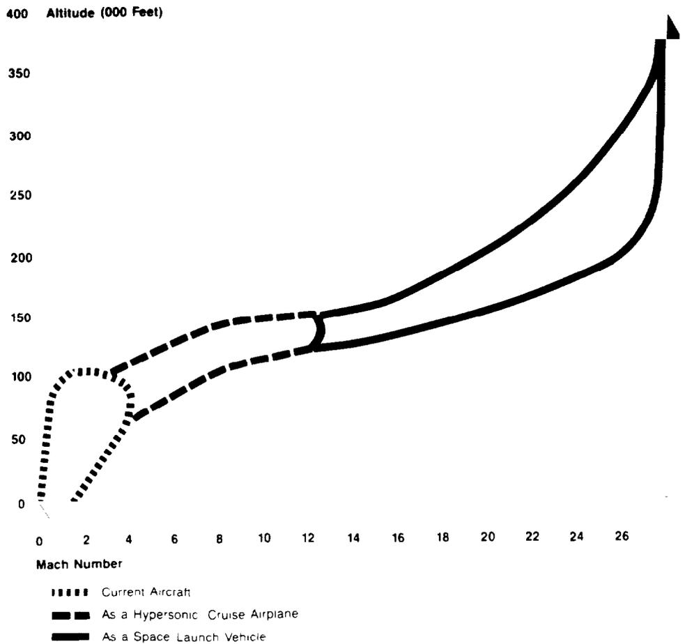
The X-30 will be designed to demonstrate sustained hypersonic cruise capability in the atmosphere at speeds between Mach 5 and 14 and at altitudes between 80,000 and 150,000 feet. Current aircraft cannot operate at these speeds and altitudes primarily due to the lack of a suitable propulsion system. The X-30 is also intended to demonstrate a single-stage-to-orbit space launch capability reaching speeds of up to Mach 25—orbital escape velocity.
