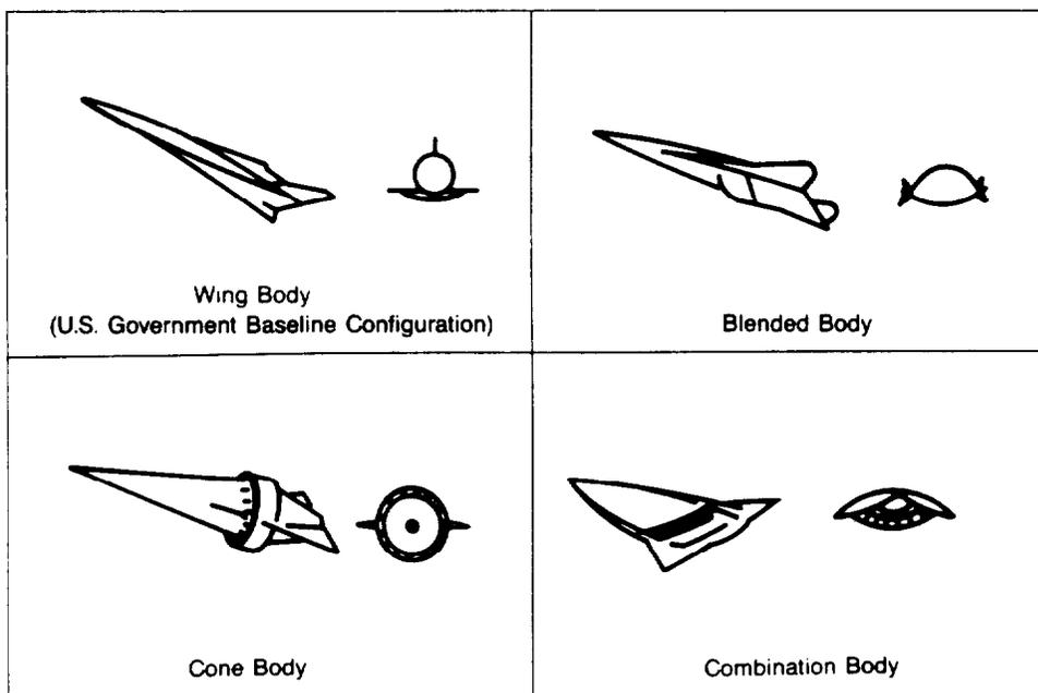
The wing body concept—the U.S. government's baseline design configuration—has a rounded fuselage and an engine that is integrated underneath the body. This configuration is aerodynamically efficient, allows
