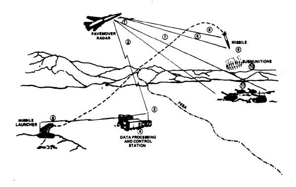
The air-launched version (fig. 2) contemplates using a B-52 or some other aircraft to launch the missile. The aircraft could also carry the radar and data processing and control station, which could provide a self-contained capability to acquire targets and to launch and guide missiles.
