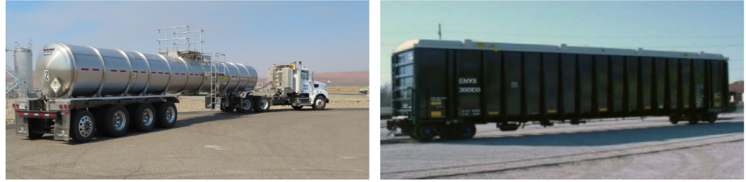
Figure 6: Transportation of Department of Energy Radioactive Waste Via U.S. Department of Transportation-Compliant Tanker Truck and Rail Car
