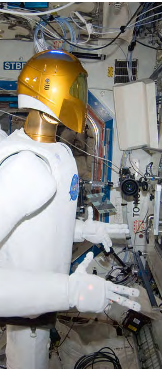
In the International Space Station's Destiny laboratory, Robonaut 2 is pictured during a round of testing for the first humanoid robot in space.
