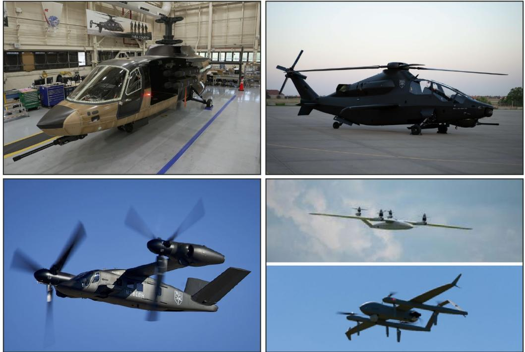
Top Row: Future Attack Reconnaissance Aircraft prototypes. Bottom Left: Future Long Range Assault Aircraft technology demonstrator. Bottom Right: Future Tactical Unmanned Aircraft System prototypes.
