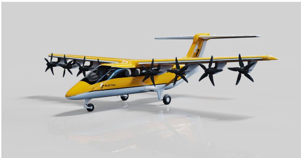
Figure 4: Electra EL9 Ultra Short, a Hybrid-Electric Aircraft with a Short Takeoff and Landing Capability
