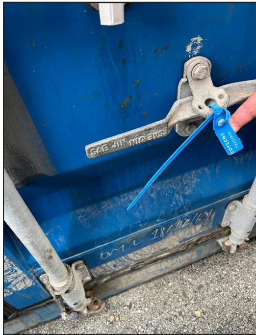
Figure 8: Example of a Container Seal Currently Used on Cargo Entering Guam
