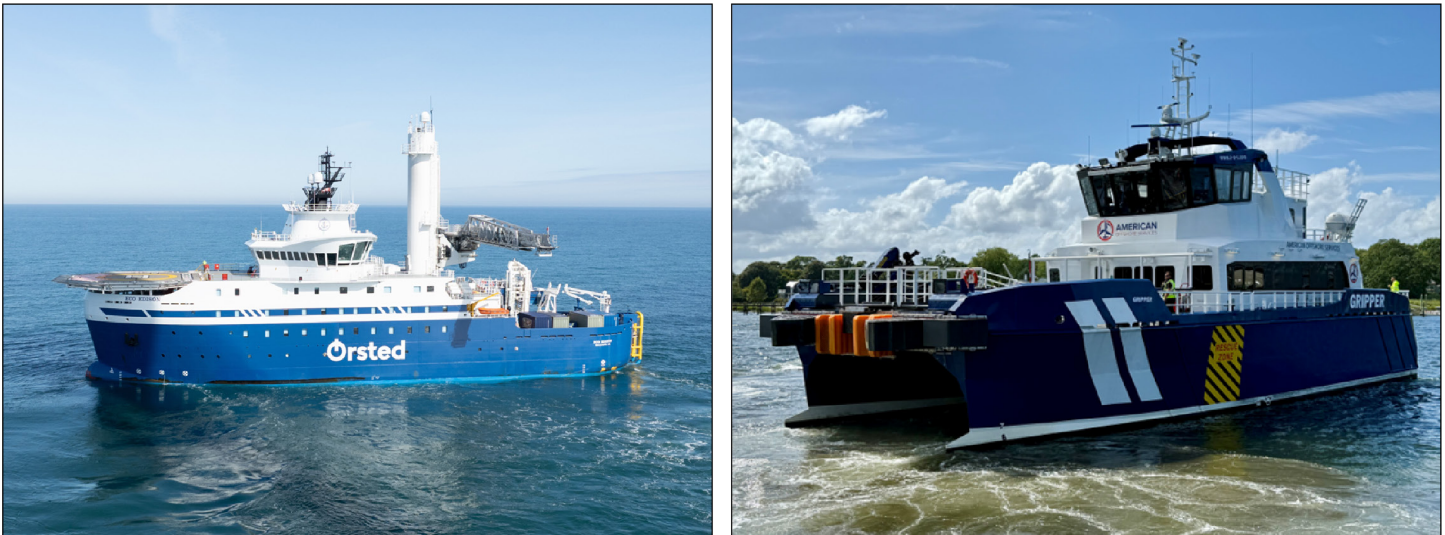
Figure 6: Examples of a Service Operation Vessel and Crew Transfer Vessel
