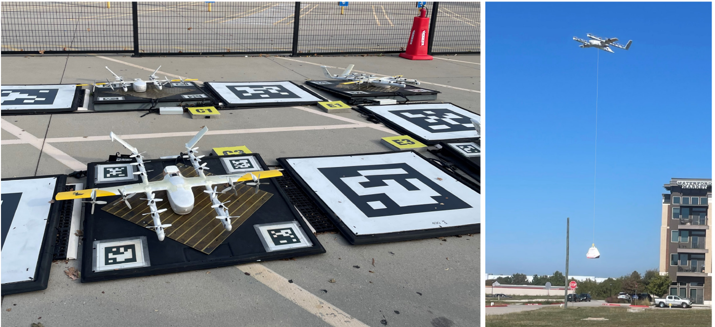
Figure 6: Examples of Drones Used for Preparing and Executing Delivery Services in North Texas
