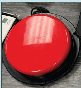
**"Red button" switch** can be connected to electronics to help students with limited motor skills use the electronics independently.
