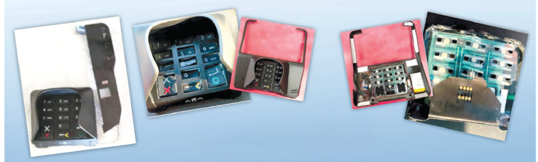
Figure 1: Sample Skimming Devices Used at Point-of-Sale (POS) Terminals
