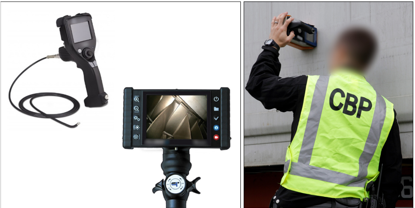
Figure 5: Videoscope (left) and U.S. Customs and Border Protection Officer Using a Handheld Density Meter to Inspect a Vehicle (right)
