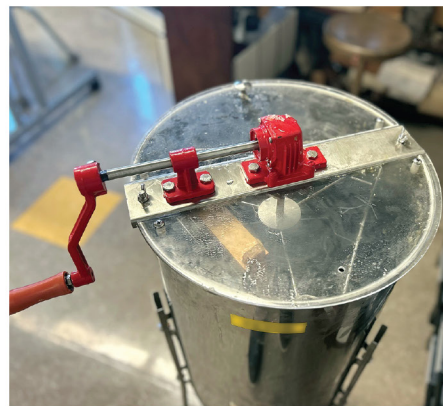
In the classroom, students cut honeycomb from the frames and use this centrifuge to extract the raw honey, learning about centrifugal force and other scientific concepts in the process.
