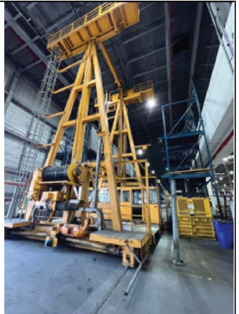
A vertical storage rack system with a lift called an elevating transfer vehicle.
