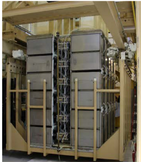
Figure 6: Photo of the Marx Bank Capacitors at Z Pulsed Power Facility, Sandia National Laboratories
