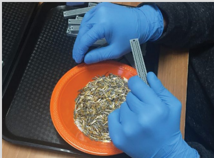
Assembly of electronic circuit pieces for airline manufacturing at a CRP.
