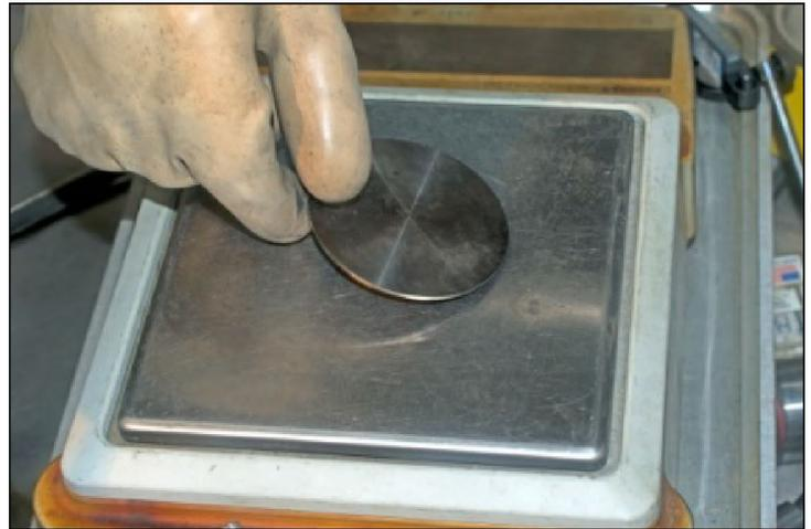
Inspecting and weighing plutonium metal sample
