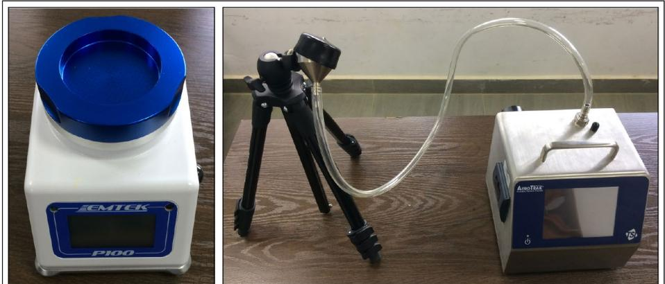
Equipment for calibrating biosafety cabinets. The Centers for Disease Control and Prevention funded training in quality control, such as calibration and maintenance of laboratory equipment.
