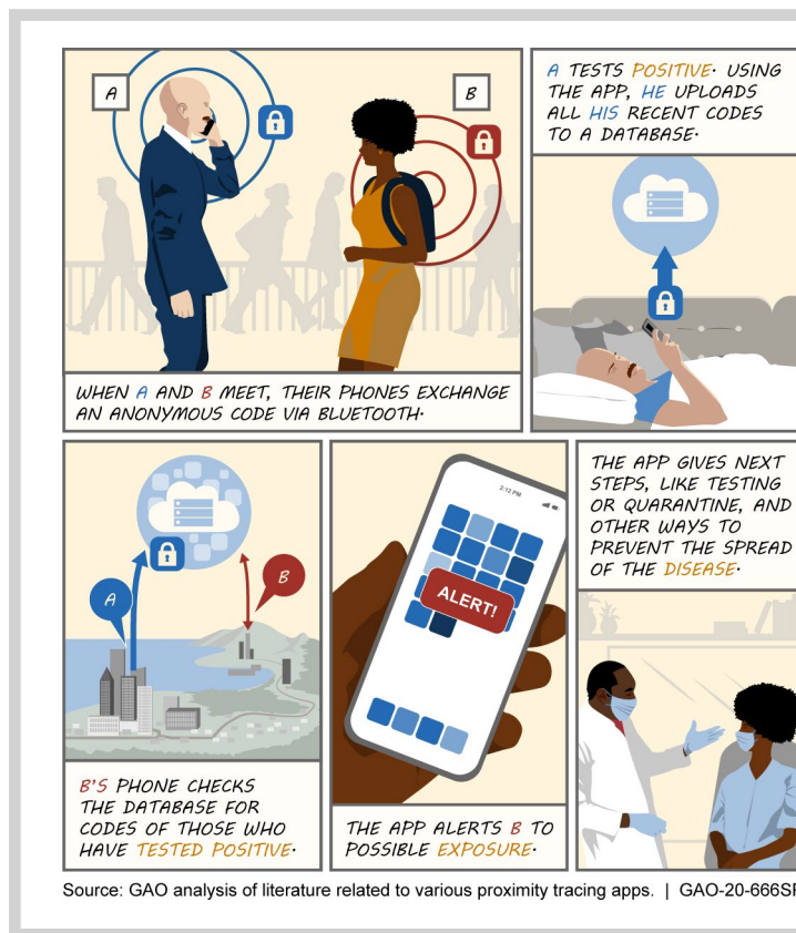
Figure 2. Bluetooth-based proximity tracing apps exchange information, notify contacts exposed to an infected person, and provide follow-up information.
