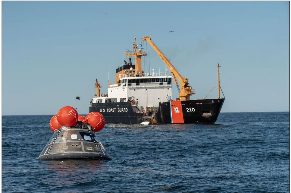
Orion program performing crew module test article uprighting tests in Gulf of Mexico with U.S. Coast Guard, U.S. Air Force, and Texas A&M University at Galveston support.
