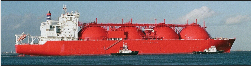
Moss style liquefied natural gas (LNG) carrier
