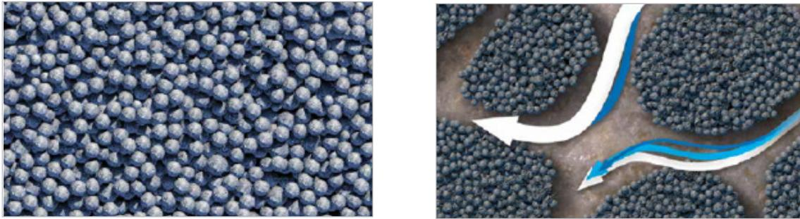
**Figure 3.2:** Flow channel creation with channel fracturing technology
