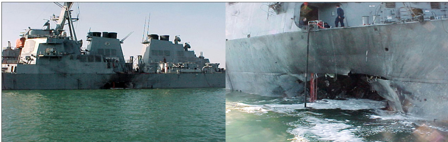
Figure 1: The Results of a Small Vessel Attack on the USS Cole
