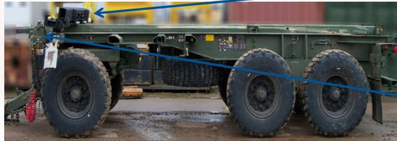
Rolling cart to allow the container to roll onto the trailer while being pushed by the CHU/E-CHU
