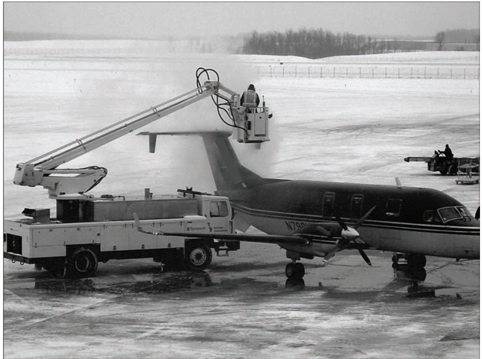
Figure 4: Example of Ground Deicing to Help Ensure Clean Aircraft
