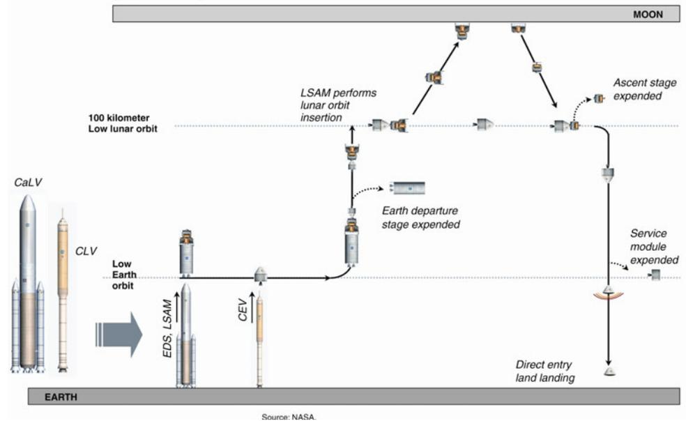
The original ESAS architecture is described below. Changes made to the architecture since the release of ESAS are described in later sections.
