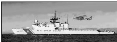
Pictured at left is a 270-foot medium-endurance cutter and an HH-65 helicopter.
