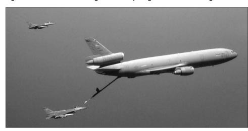
Figure 1: KC-10 Aerial Refueling Aircraft Preparing to Refuel an F-16 Fighter
