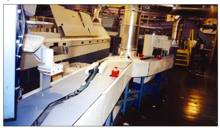
Figure 6: DBCS Modified with Plastic Shrouds
