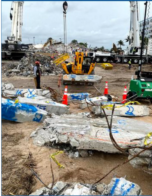
Building elements such as columns, beams, and floor slabs identified for evidence review (July 2021)
