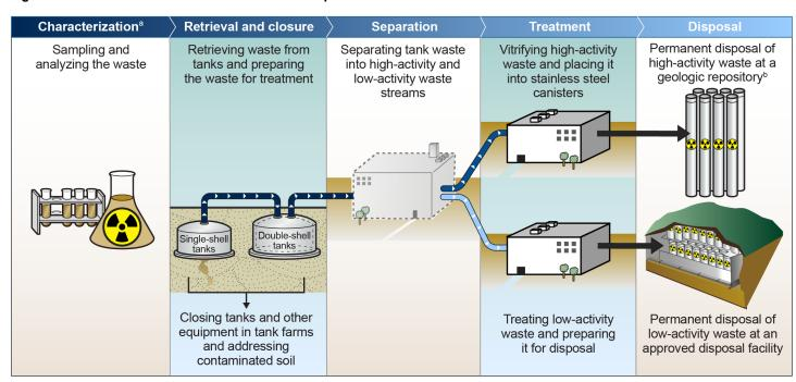
Figure 1: Phases of Tank Waste Treatment and Disposal at the Hanford Site
