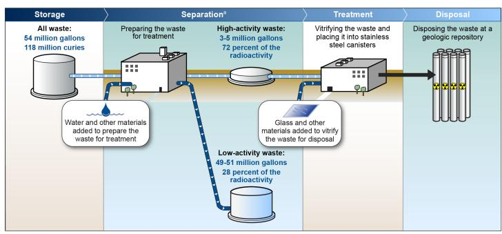
Figure 4: Department of Energy's Current Plan for Treating the Tank Waste at the Hanford Site
