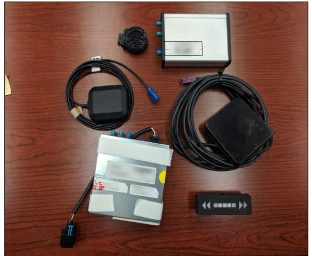
This equipment – used by the Ann Arbor Connected Vehicle Test Environment – allows connected vehicles to wirelessly communicate with each other and their surrounding environment. The vehicle's equipment transmits speed and position data to other research equipment located roadside, in other vehicles, and at intersections.
