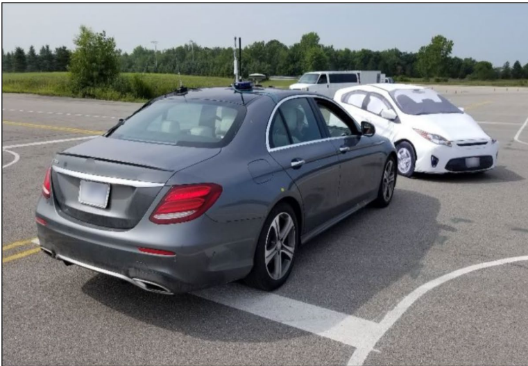
Crash avoidance test with an advanced driver assistance system using robotic control testing equipment.
