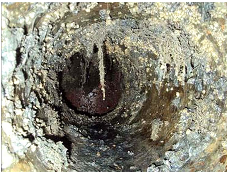
Figure 6: Biofouling Inside a Pipe on an LPD 17 Class Ship
