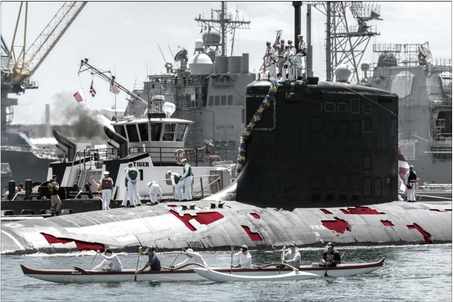
Figure 7: SSN 774 Class Submarine Returning from a Deployment with Missing Special Hull Treatment
