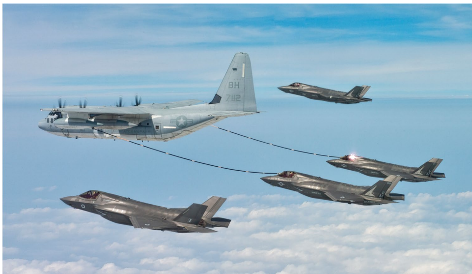
Figure 8: F-35B Aircraft Refuel from a KC-130 Aerial Refueling Tanker Using Hose and Drogue Refueling Equipment
