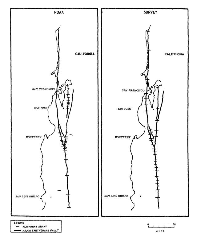
LOCATION OF ALIGNMENT ARRAYS OF NOAA AND THE SURVEY APRIL 1971
