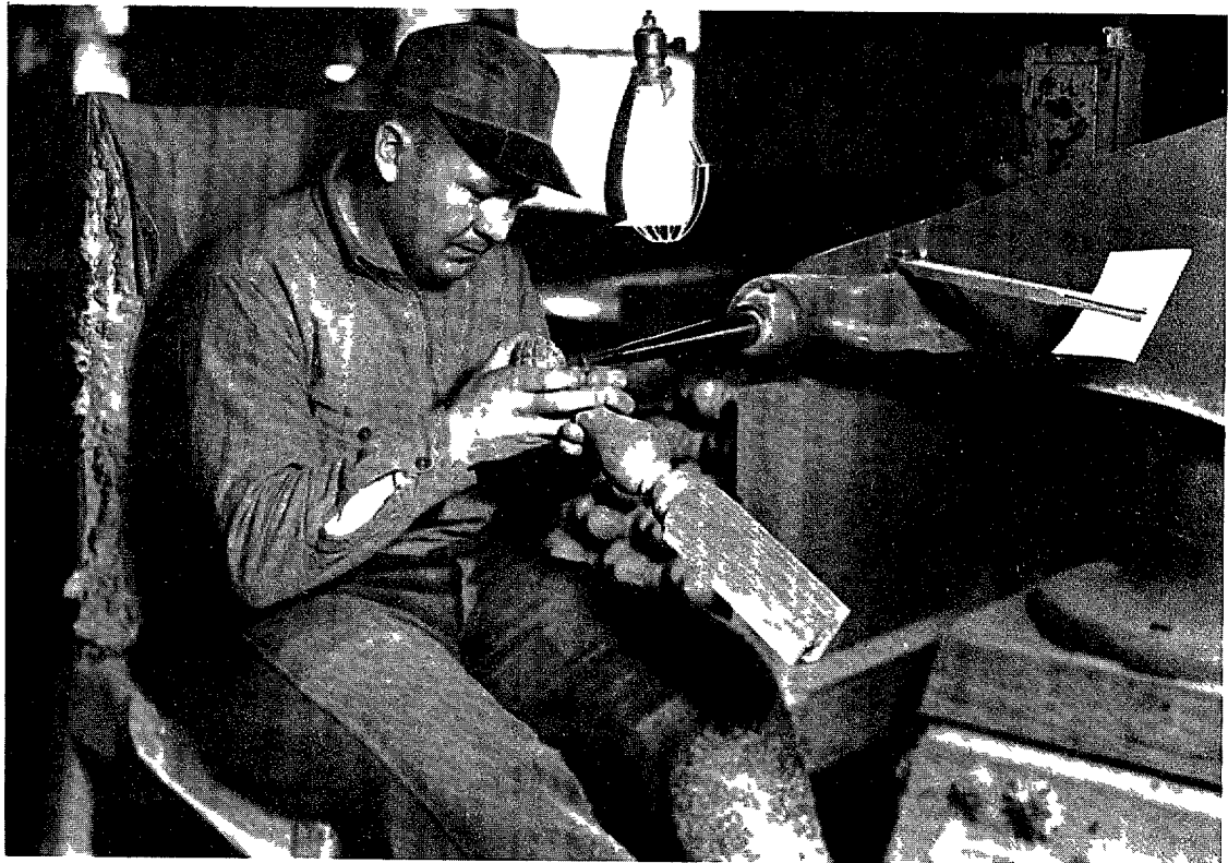
A 4 Worker using spindle sander is exposed to respirable wood dust particles
