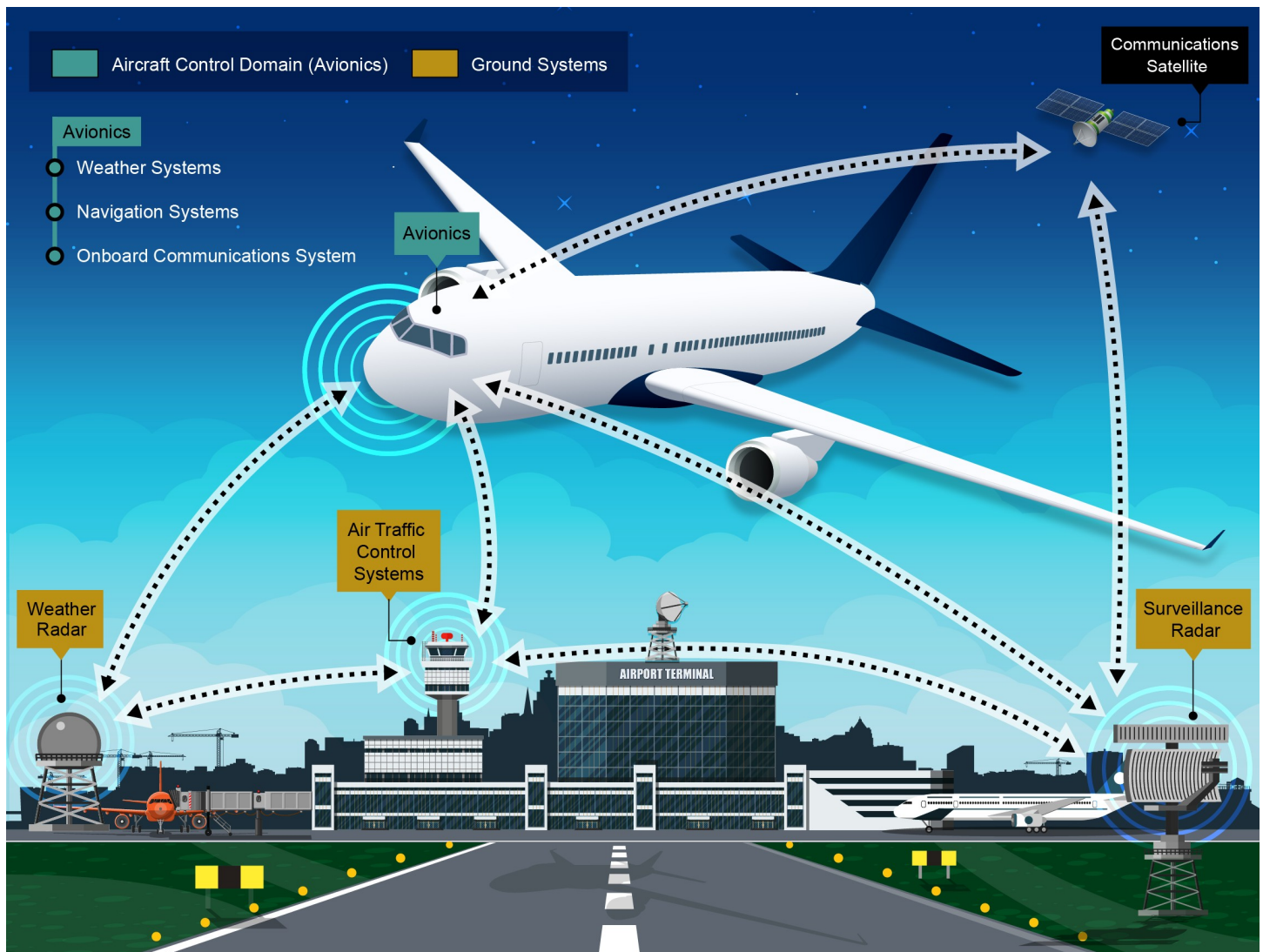
Figure 3: Interconnected Avionics and Ground Systems That Support the National Airspace System
