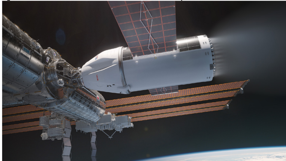
Figure 4: The U.S. Deorbit Vehicle Docked to International Space Station
