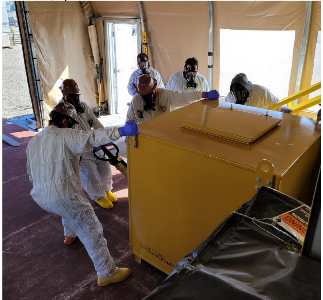
Figure 4: A Shipment of Liquid Low-Activity Waste in a Double-Walled Steel Container is Prepared at the Hanford Site, May 2025
