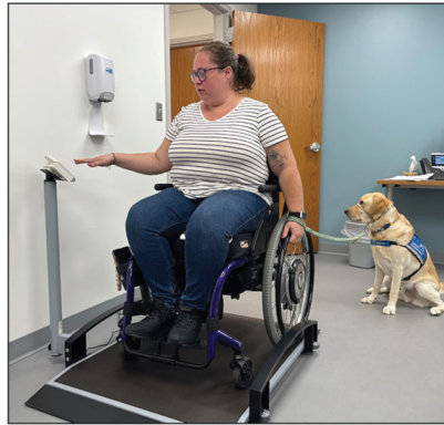
A patient using a wheelchair scale. A person in a wheelchair will have their chair weighed separately, then be weighed while sitting in the chair, allowing providers to obtain their accurate weight.
