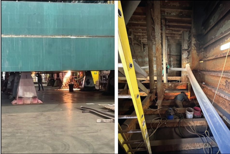
Figure 2: Images of a Shipyard Worker Welding Steel Plates into a Block (left) and Welding Inside a Vessel During a Repair at a U.S. Shipyard (right).
