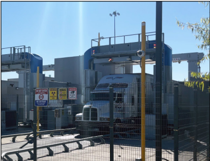
Multi-energy portals scan commercial tractor trailers.
