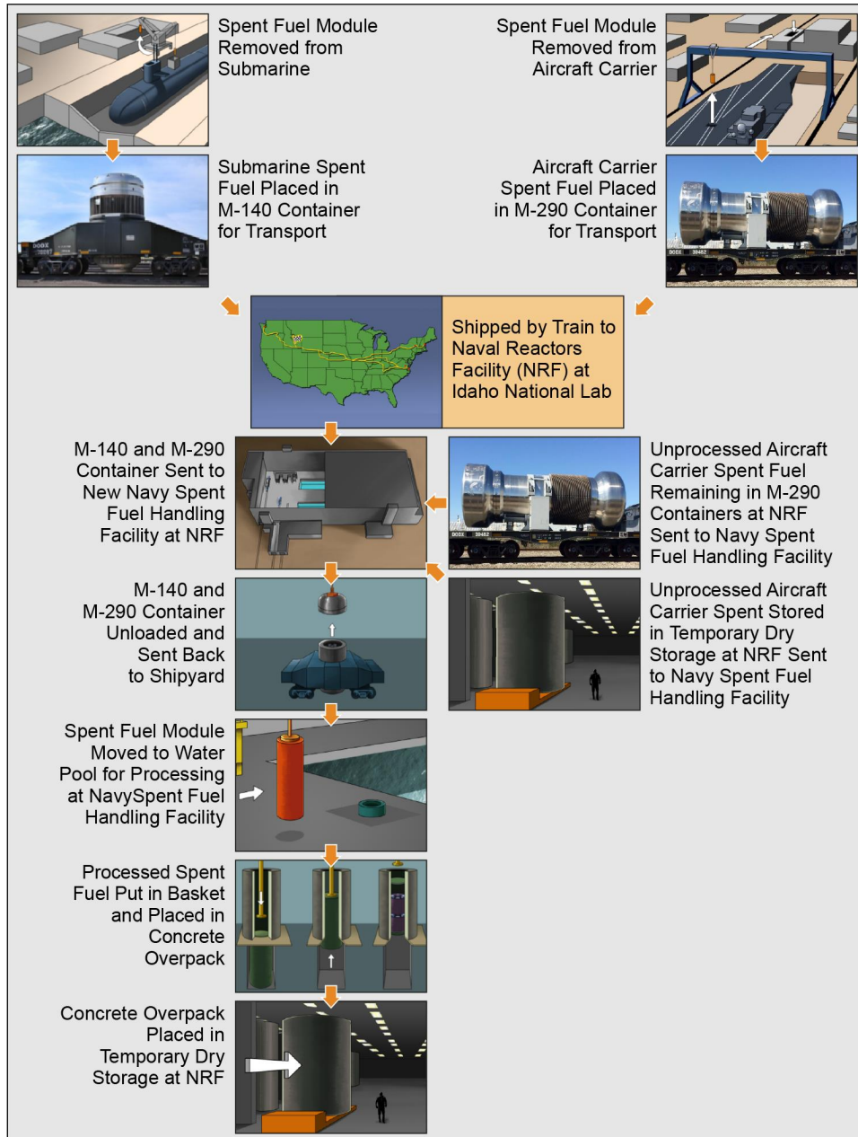
Figure 5: Future Process for Managing Naval Spent Fuel with the Spent Fuel Handling Facility
