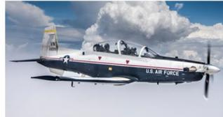
**T-6A Texan II** is a single-engine, two-seat primary trainer designed to train entry-level students in the fundamentals of flying.
