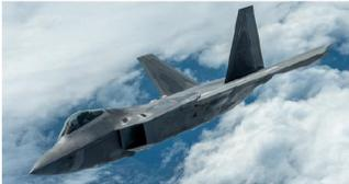
**F-22A Raptor** is a fifth-generation fighter aircraft designed to engage air targets at great distances and is air-to-ground capable.
