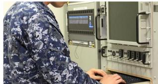
**Navy Multiband Terminal (NMT)**—installed on ship, shore, and submarine platforms—enables communication with satellite systems using various frequency bands, communications protocols, and data rates.
