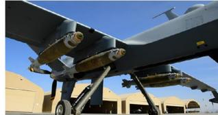
**Joint Direct Attack Munition (JDAM)** is a GPS-guided kit attached to conventional bombs to increase weapon accuracy.
