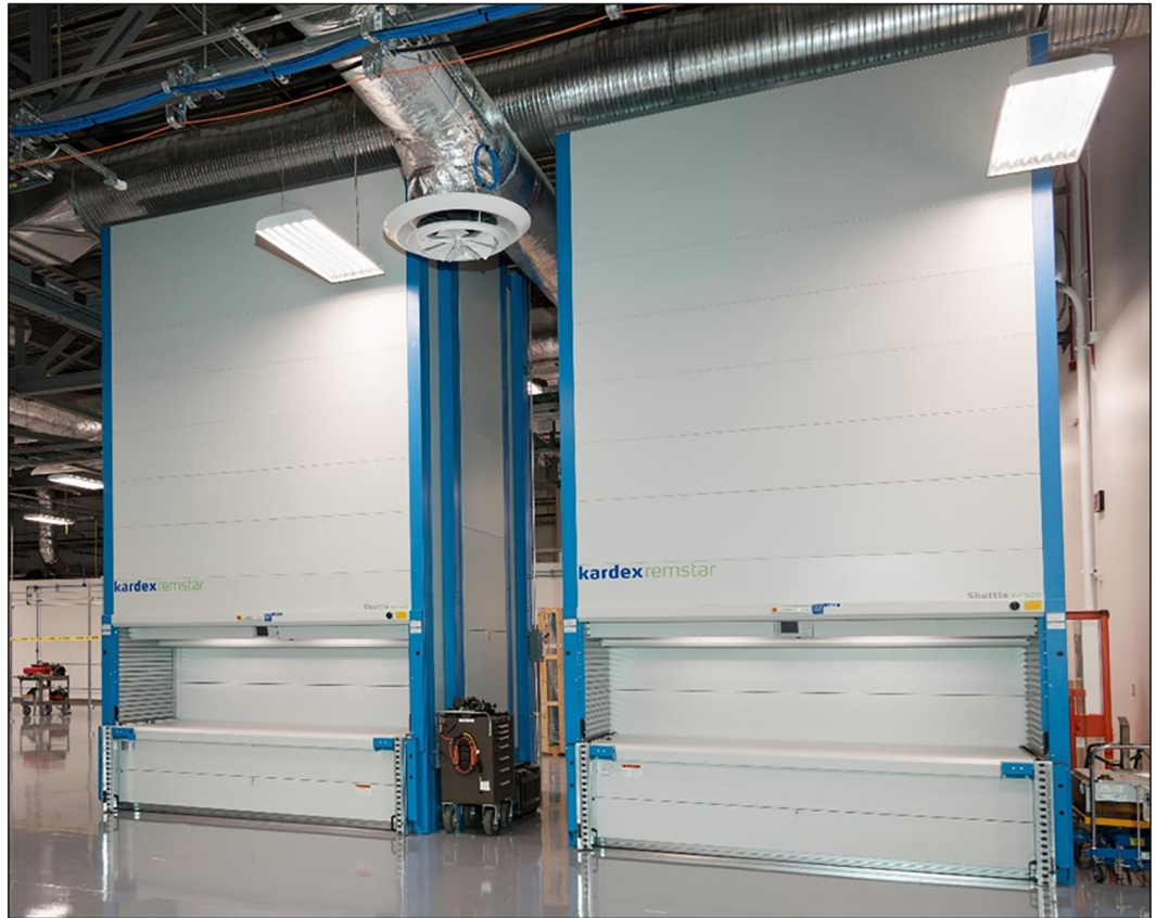
Figure 4: Vertical Equipment Storage Systems at the Kansas City Site
