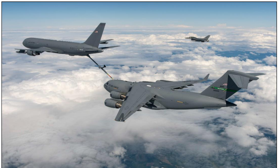
Figure 2: KC-46 Aircraft Using a Boom to Refuel a Receiver Aircraft
