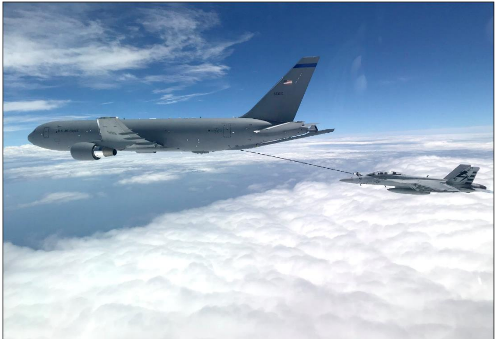
Figure 3: KC-46 Aircraft Using the Centerline Drogue System to Refuel a Receiver Aircraft
