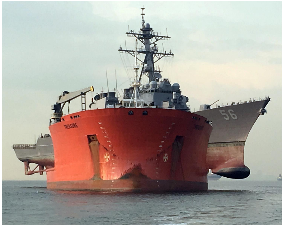
Figure 3: USS John S. McCain Transported aboard the MV Treasure after Its 2017 Collision
